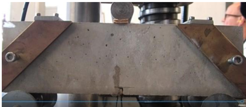
Figure 4 Healing of a crack due to flow through an internal vascular network [26]
